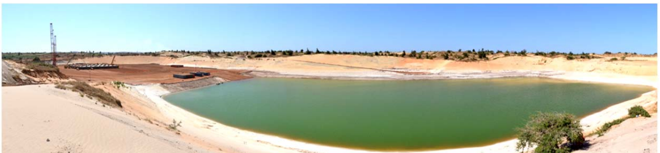
Completed dredge start pond, with beginnings of wet concentrator plant (WCP) in background
